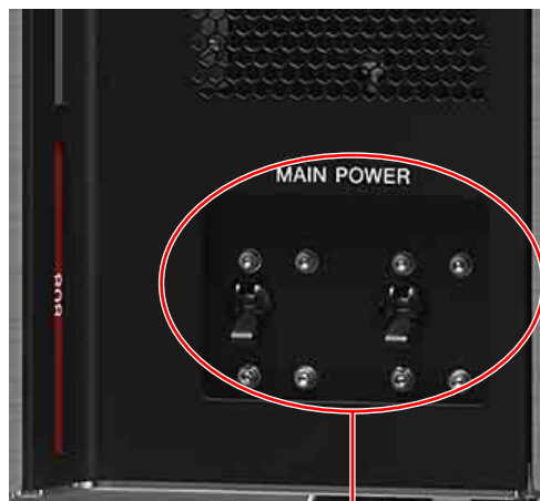
Main power switches
